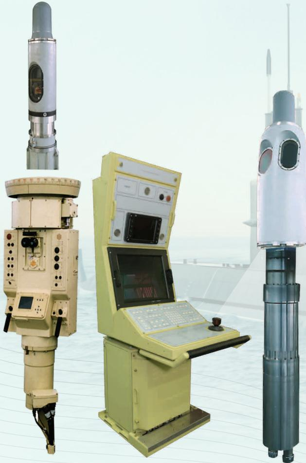
Unified Periscope System PARUS-98E consists of attack periscope penetrating into the submarine hull and multipurpose non-hull-penetrating periscope (optronic mast). The periscope complex can be supplied as a complete set or separately
