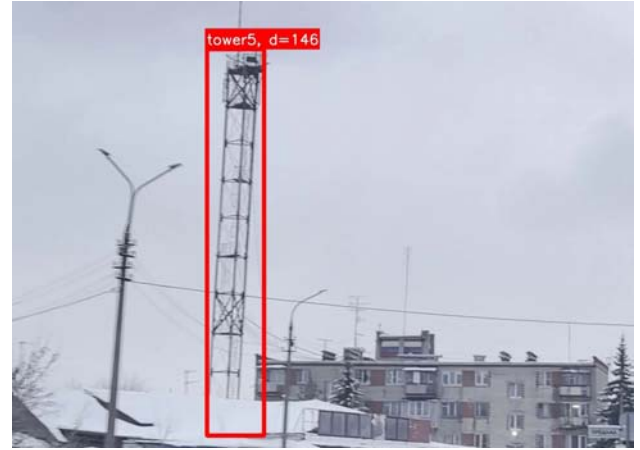
Fig. 5. Landmark detection, classification and distance determination.
