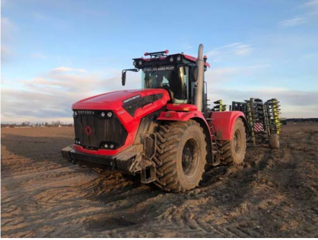
Fig. 2. Kirovets K-7M with the Cognitive Agro Pilot system
