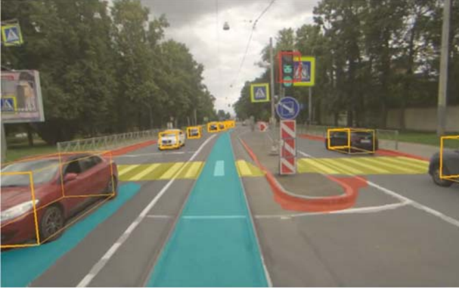
Figure 2. Visualization of road scene recognition (3D detections - cars (yellow), traffic lights (red), segmentation area - curbs (red), tramway (turquoise))
