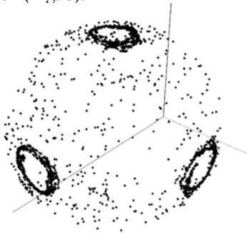
Fig. 8. Magnetic field sensor readings during rotation around three axes
